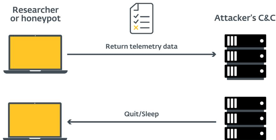
Figure 12 // Researcher machine (honeypot) reports artificial telemetry data to the attacker's C&C, receives sleep/quit command.
